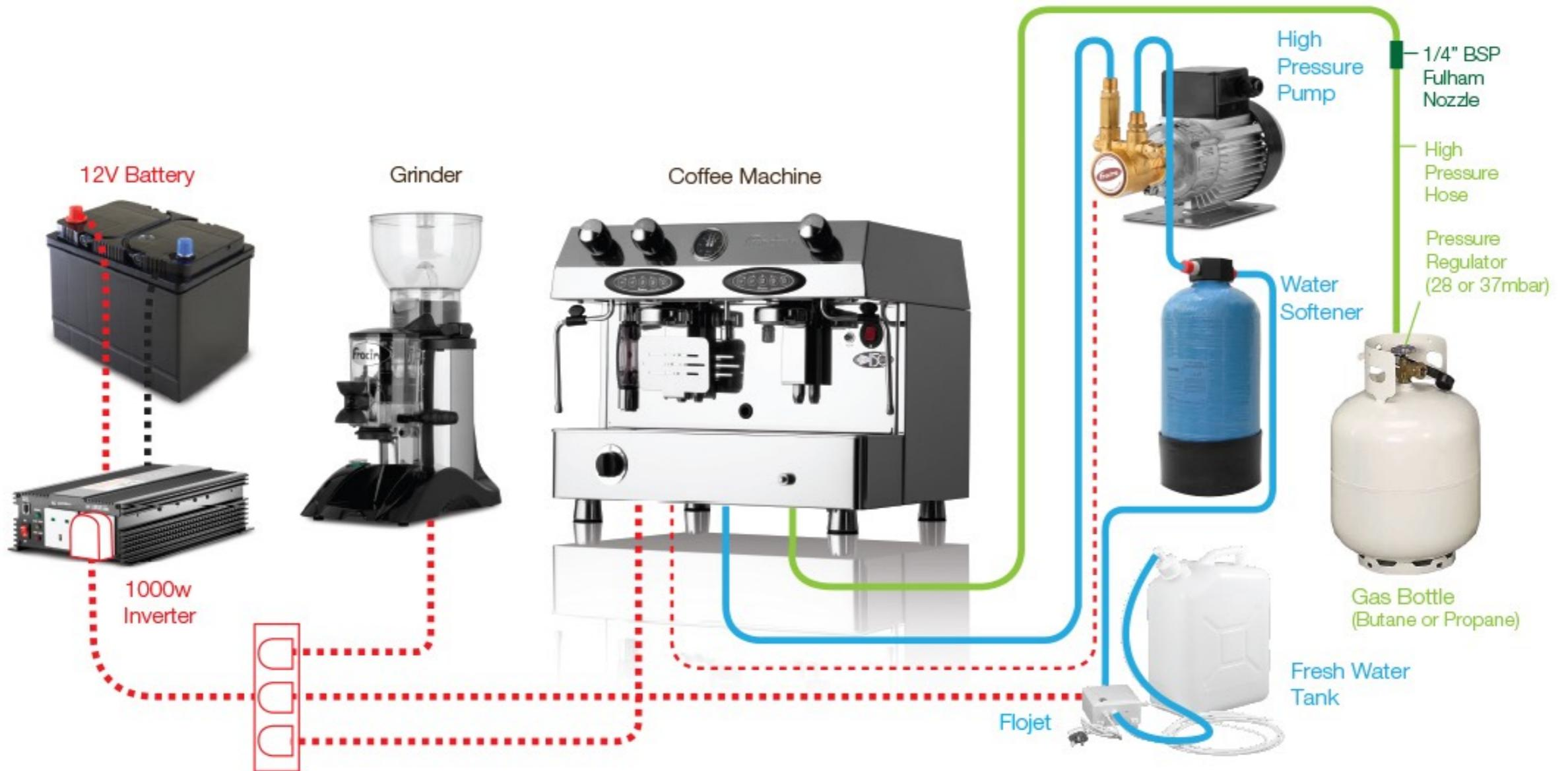
Key: ..... Power Supply — Water Supply — Gas Supply
